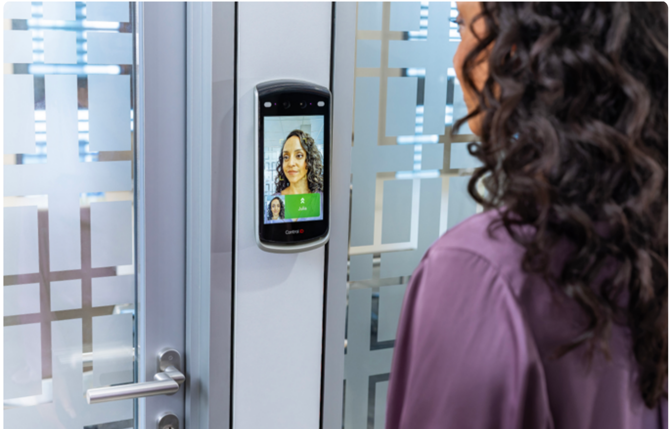
Control iD biometric readers can be used as a stand-alone access control system or integrated with other systems, such as Impro Primo
