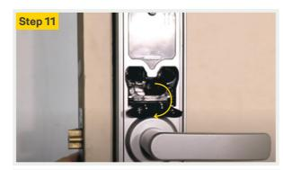
Push in and slide down on the battery tab as shown in the image to open the battery compartment. Install the 4 x AA Alkaline batteries. \*Carefully note the indicated "+" & "-" pattern shown on battery compartment. Once the batteries are installed, test the latch retracts when turning both internal and external levers.
