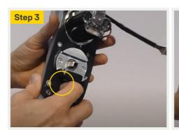
To hand the lock, hold down on the metal slide tab and rotate the handle left or right depending on your selected handing. Ensure you hold down the tab at all times during the rotation. Rotation should be smooth, if you experience firm resistance, release the handle and slide tab and repeat handing process. Ensure you complete this for both handles.
