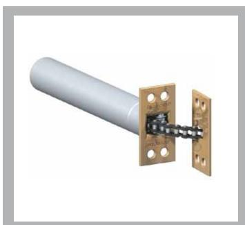
The Interlock Securicloser provides automatic closure of timber or aluminium doors fitted with standard hinges. The closing power is adjustable without removing the unit from the door and can be set to door size and weight. The Securicloser is strong, durable, hidden from view and fits most standard doors.
