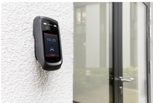
Control iD biometric readers can be used as a stand-alone access control system or integrated with other systems, such as Impro Primo
