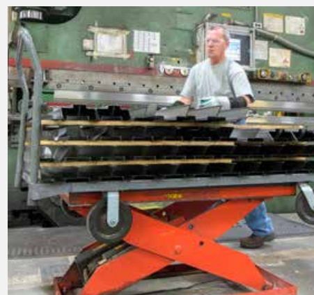
Lifting equipment adjusts working height to a comfortable level to prevent the operator from having to bend over.
