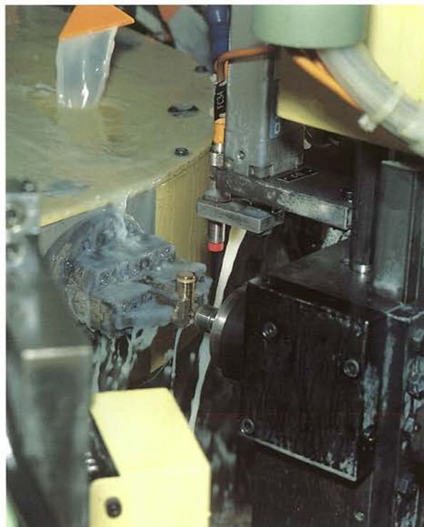
A Computerized Numerical Control machine center for the production of cylinder cores.
