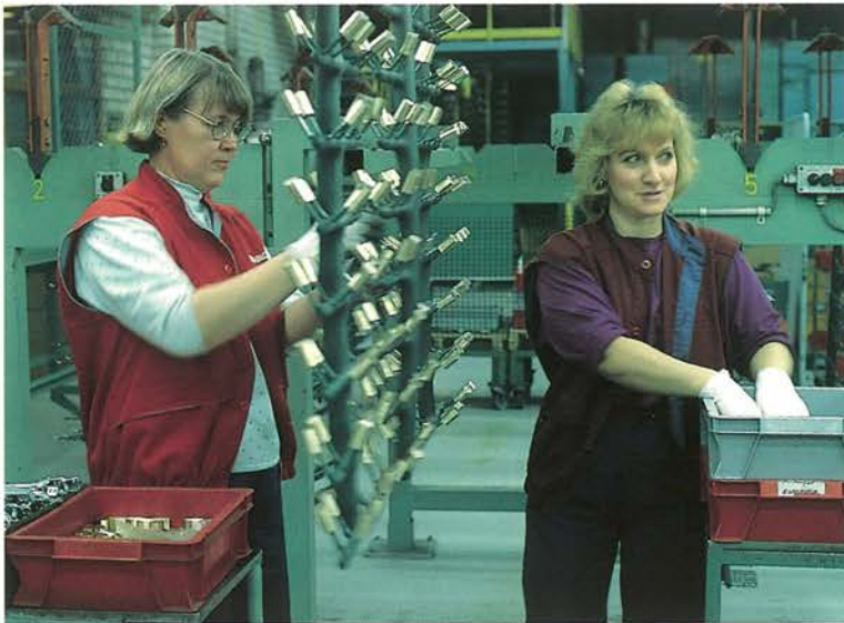
Surface finishing of padlocks in the ABLOY plant.
