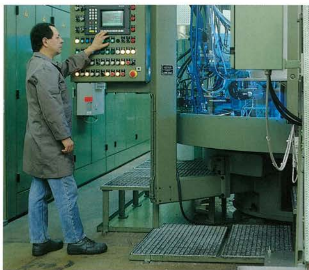
CNC-automatic machine for manufacturing of cylinder cores.
