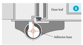
The asymmetrical mounting bracket is attached to the frame
