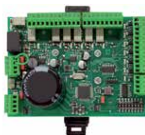
Evaluation control unit without housing, on mounting rail adapter
