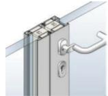
This system is a highly advanced thermally insulated profile system used for flush mounted single or double-leaf swing doors, single and double-leaf sliding doors, windows and glazed partitions.
