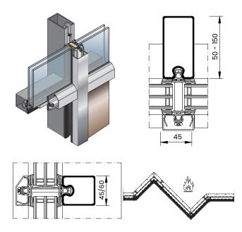
Thermfix Vario is the system for thermally insulated, internal and external grade, curtain walls and skylights comprising of mild steel profiles, stainless steel pressure plates and aluminium or stainless-steel cover caps.
